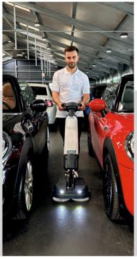
The compact scrubber-dryer machine is the ideal mechanical alternative to mopping systems and can be used on all type of floor coverings. The combination of two rotating brushes or pads with the powerful suction motor ensures a dry and streak-free surface that can be walked on immediately.
